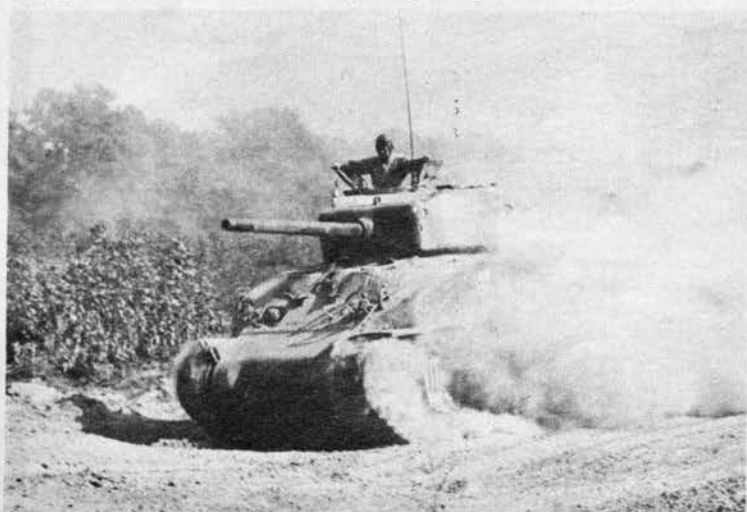
Short, fat assault gun on the Sherman tank is a 105-mm. howitzer. Long-barreled gun below is a high-velocity 76-mm. which calls for a bigger turret with roomier fighting compartment, larger hatches.
